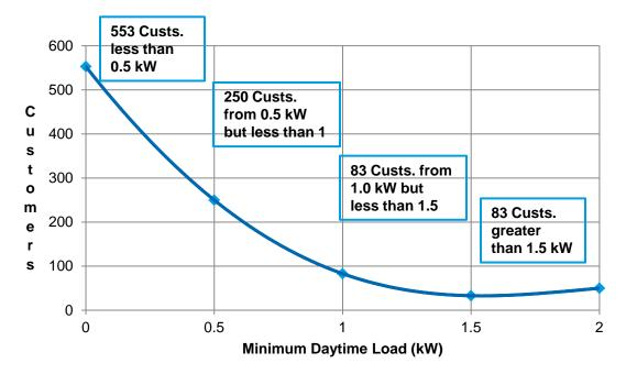
The above analysis shows that at MDL, during high solar output hours, the customer load can be extremely low. This means that most of the solar at that point in time will be exported into the system. This not only causes voltage rise at the customer site, but can also cause voltage rise on the distribution circuit and, for large enough concentrations, on the transmission system.
