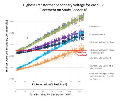
Figure 20: Mitigation Options for Feeders with High Voltage due to Presence of PV
