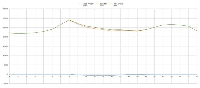
Figure 11: Comparison of Gross Load to PV Generation on a Pepco Feeder (Hour of Day vs. kW) for a Winter Peaking Feeder
