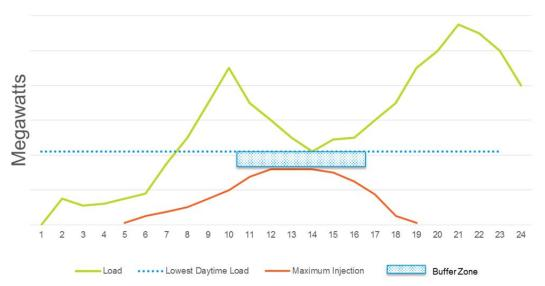
Note that Figure 6 is illustrative and that every feeder on the PHI system will have a different composition of customer load and generation. Generally, however, most feeders experience periods of low customer load and high customer generation, as depicted in this chart, on the weekends in the spring and fall seasons.
