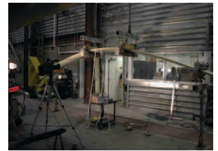
Bergey WindPower blade testing
