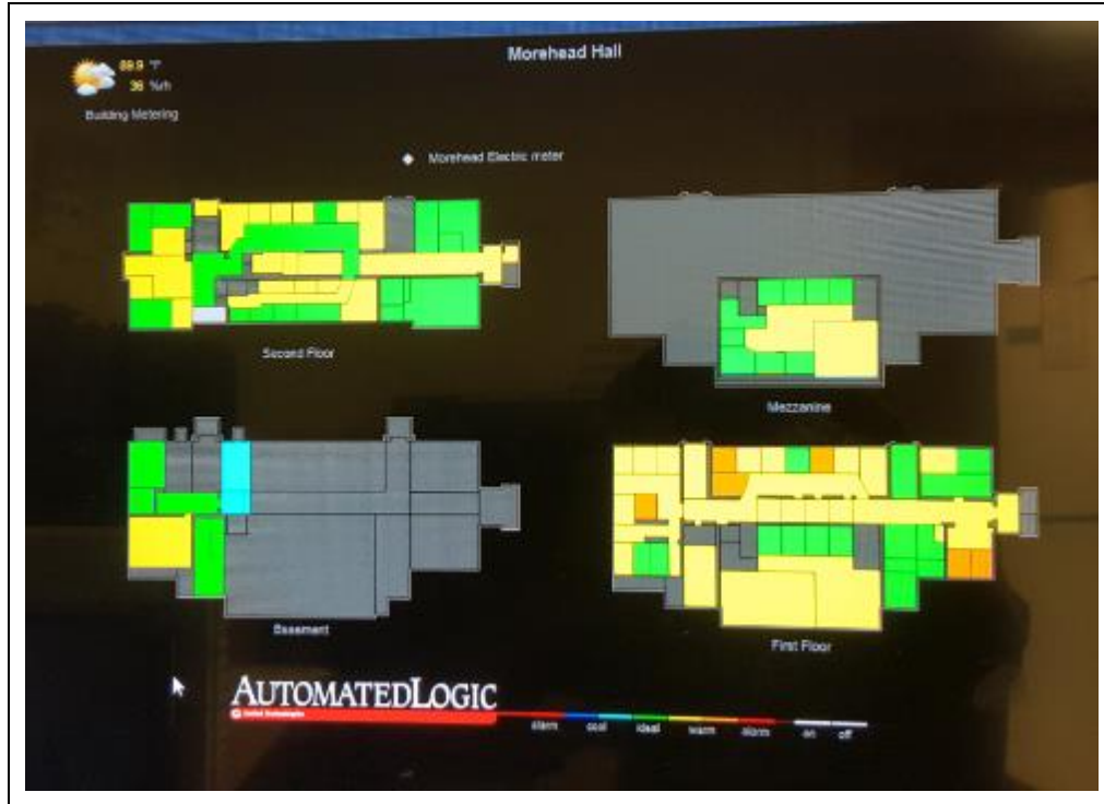
Figure 10 – Building Energy Management System (BEMS)
