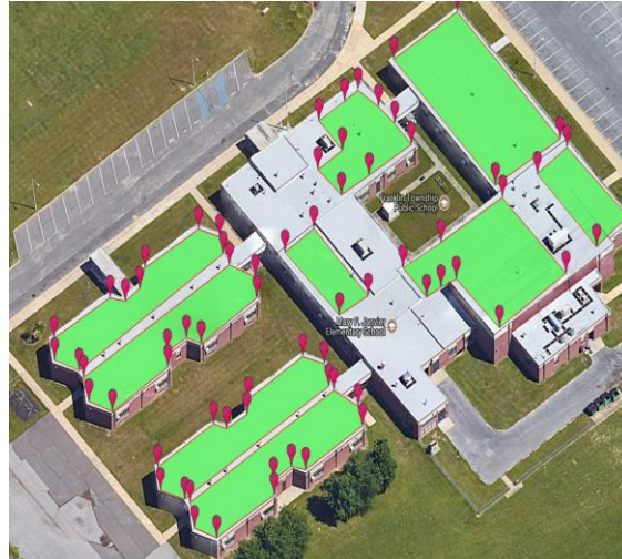
Figure 22 Identified roof areas for solar panel installation
