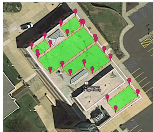
Figure 25-Potentially Available Rooftop Spaces for Solar PV Development at the Library
