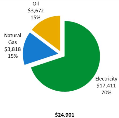
An energy balance identifies and quantifies energy use in your various building systems. This can highlight areas with the most potential for improvement. This energy balance was developed using calculated energy use for each of the end uses noted in the figure.
