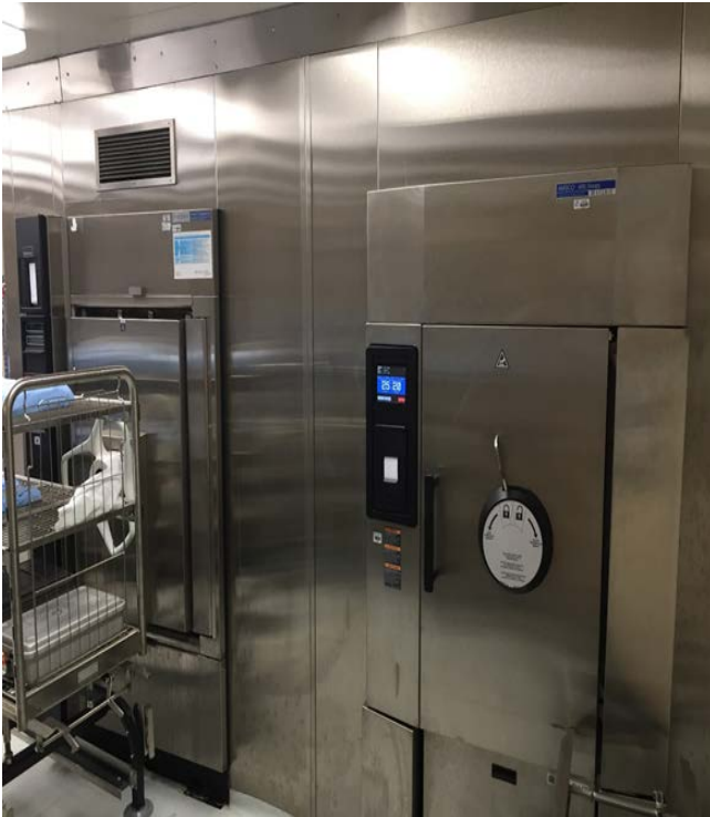
Image 13: Amsco 300 & 400 Series Sterilizers & Steam Jacketed Chamber
