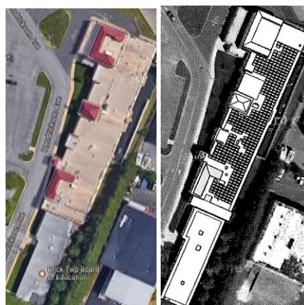
Image 8: School's rooftop before and after solar PV installation
