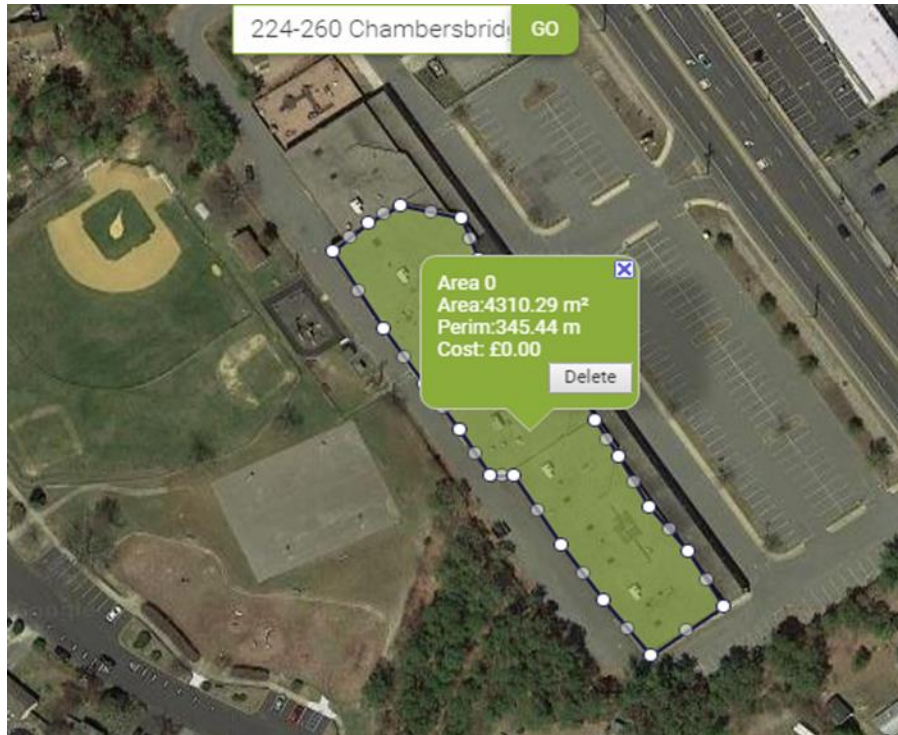
Figure 22- Warren H. Wolf Elementary School Rooftop (approximate size of proposed solar PV array)
