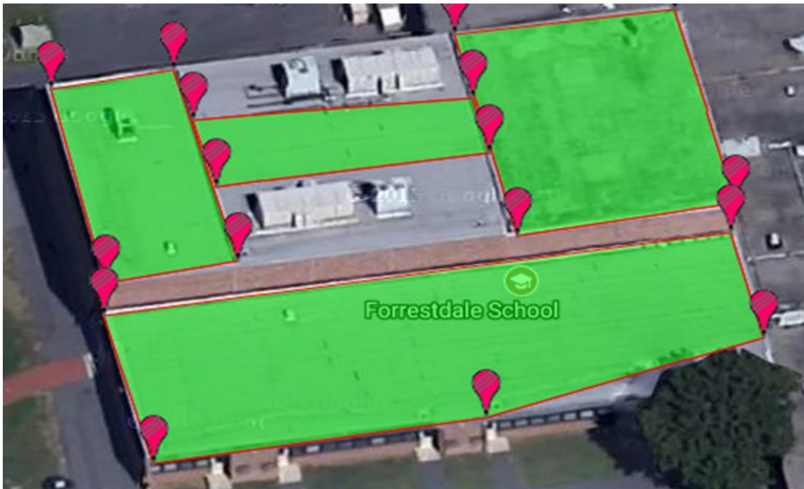
Roof Top Free Area for PV installation
