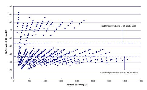
Figure 6 Air Cooled Condenser Specific Fan Power as a Function of Condenser Size
