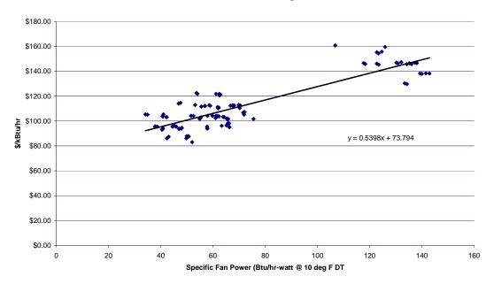
Figure 8 Air Cooled Condenser Cost Correlation
