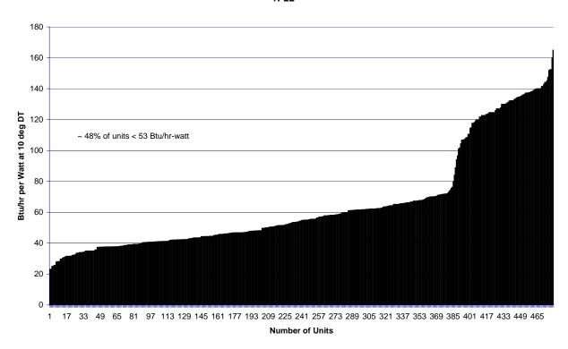
Figure 5 Air Cooled Condenser Specific Fan Power Distribution
