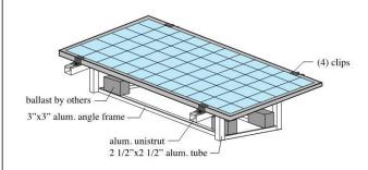
RACKING ROOF SOLAR SYSTEM assambly SLOPE 10°
