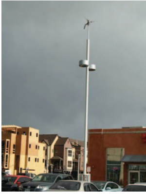
Southwest Windpower "Air" on lamppost
