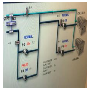
Newer Wing Chilled Water Control Loop
