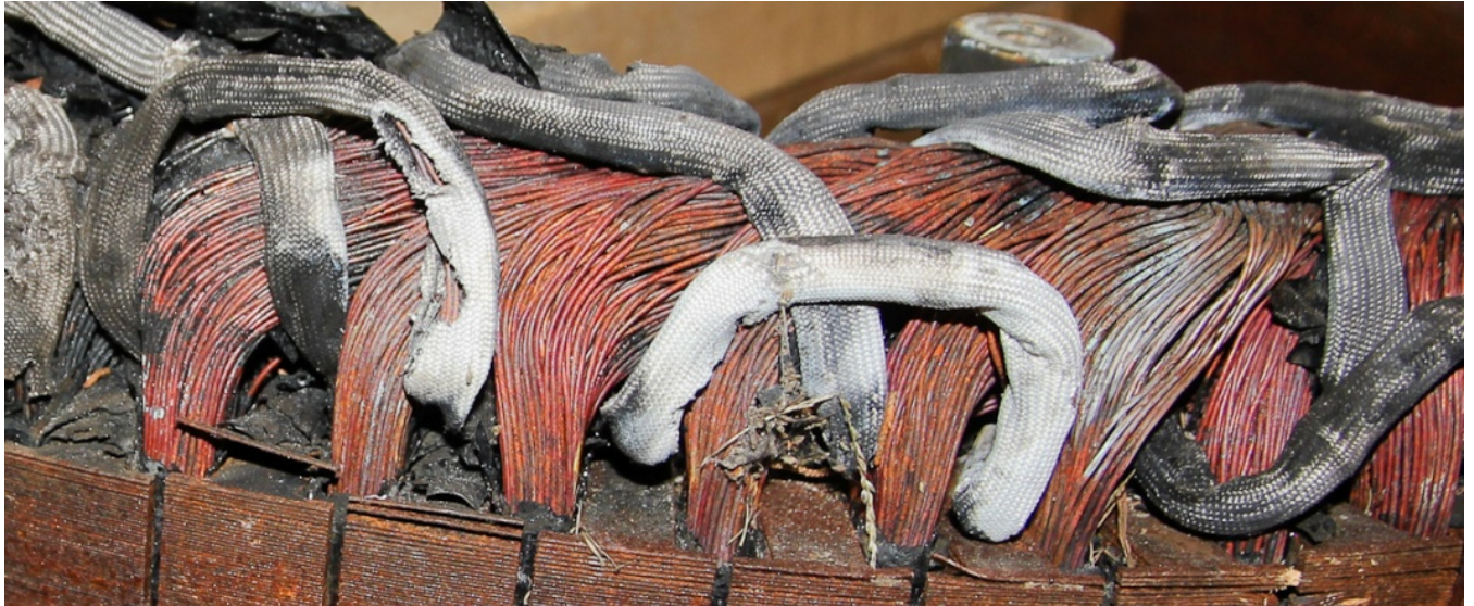
Figure 14. Alternator stator windings with the varnish burned off (Photo by Lee Jay Fingersh, NREL)
